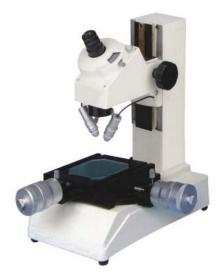
iMeas-505 is widely used in mechanical, meter, electronic and light industry; university, Institute and metrology department. The measuring profile projector can detect the contour dimension and surface shape of variety complex workpiece, such as templates, punching pieces, cams, threads, gears, molding milling cutters.
